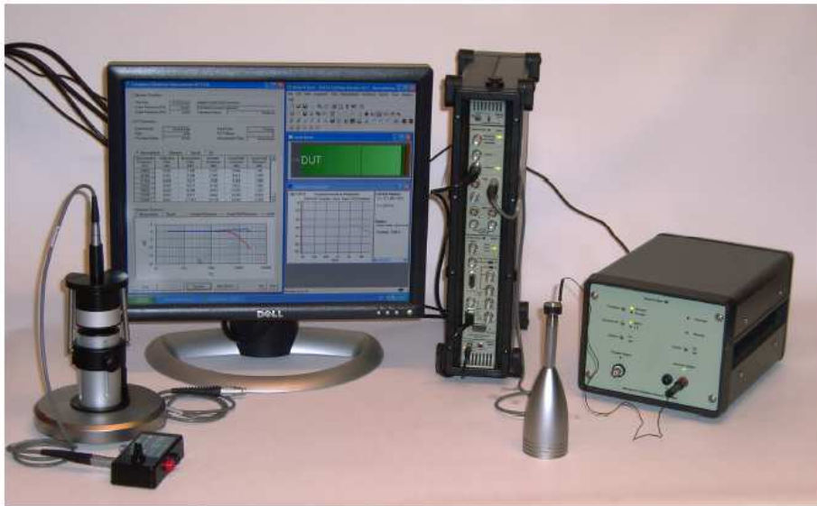
Microphone Calibration System Type 9721 with its PULSE Analyser, its Sensitivity Calibration Coupler Stand (left) and its Electrostatic Actuator Setup (right)
