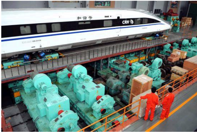
Test platform for 600km/h operation speed
