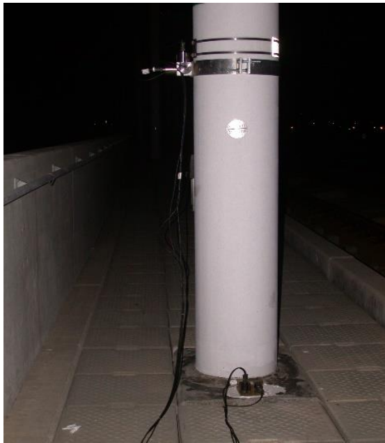
Sensor mounting position for natural frequency measurement
